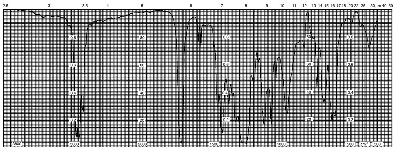
**Figure 26.** IR transmission spectrum recorded from a “phthalate plasticized” PVC. [Reproduced from spectrum number 2018 in ‘Atlas of Polymer and Plastics Analysis’, 2nd edition, Vol. 2, Part a/I, D.O. Hummel, Verlag Chemie GmbH, Weinheim (1984).]
