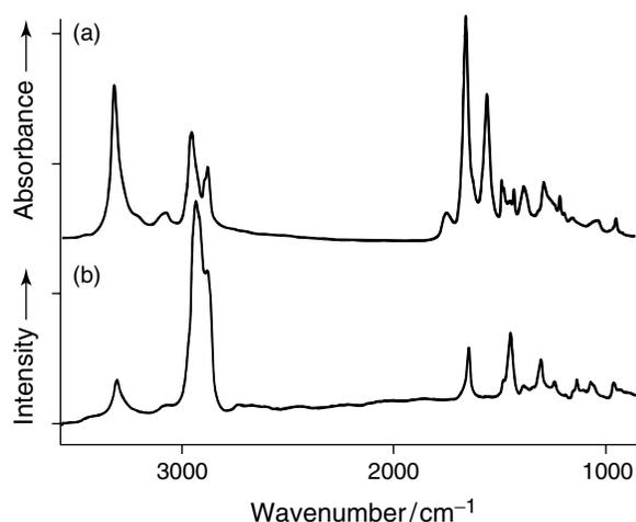
**Figure 6.** (a) IR absorbance and (b) Raman spectra of Nylon 6, 6. [Reproduced from J.M. Chalmers and N.J. Everall, Chapter 4, ‘Vibrational Spectroscopy’, pp. 69–114, in ‘Polymer Characterisation’, eds B.J. Hunt and M.I. James, Blackie Academic & Professional, Glasgow (1993).]
