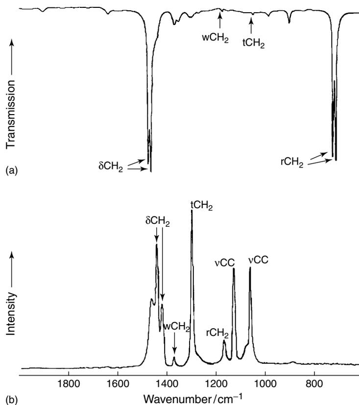
**Figure 2.** (a) IR transmission and (b) Raman spectra from 2000 to 600 cm<sup>-1</sup> of PE (w, wag; v, stretch; δ, deformation; r, rock; t, twist). [Reproduced, with permission, from H.A. Willis, 'Combination of Spectroscopic Methods in Polymer Structure Analysis', in "Proceedings of 5th European Symposium on Polymer Spectroscopy", ed. D.O. Hummel, Verlag Chemie, Weinheim (1979).]
