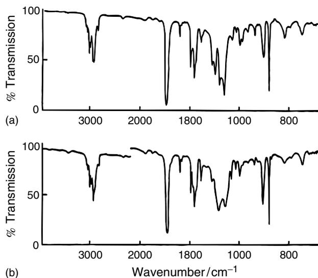
**Figure 24.** IR transmission spectra of methyl methacrylate/styrene copolymers: (a) a “block” copolymer; (b) a “random” copolymer.
