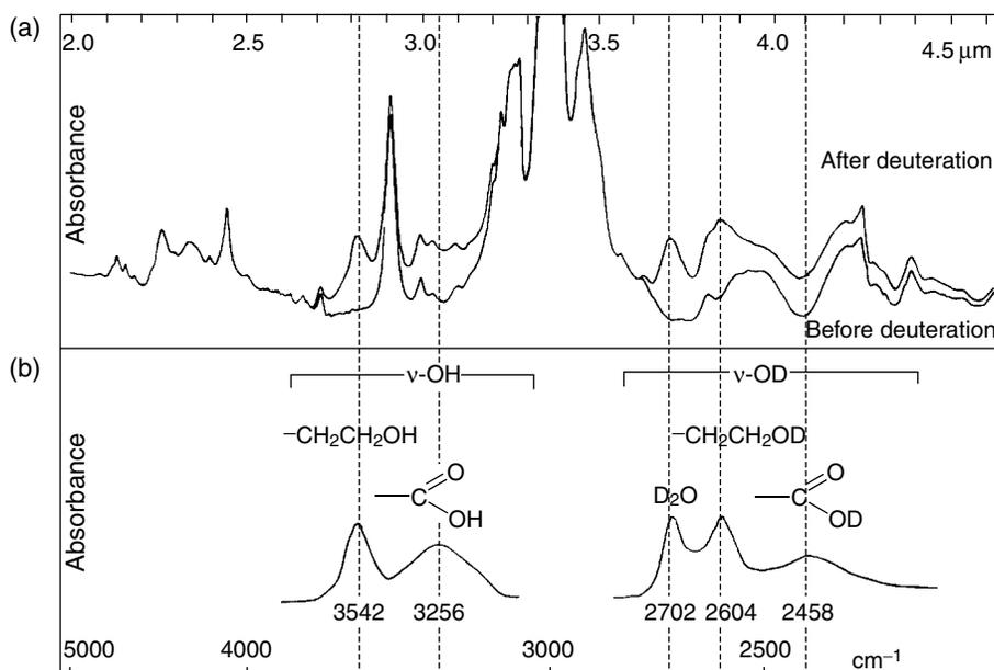
**Figure 11.** (a) IR absorbance spectra of a dried PET film before and after exposure to  $D_2O$ . (b) Difference IR absorbance spectra between PET film spectra before and after deuteration. [Reproduced from J.M. Chalmers, 'Infrared Spectroscopy in Analysis of Polymers and Rubbers', in "Encyclopedia of Analytical Chemistry", ed. R.A. Meyers, 7702–7759, Vol. 9 (2000). © John Wiley & Sons, Ltd. Reproduced with permission.]
