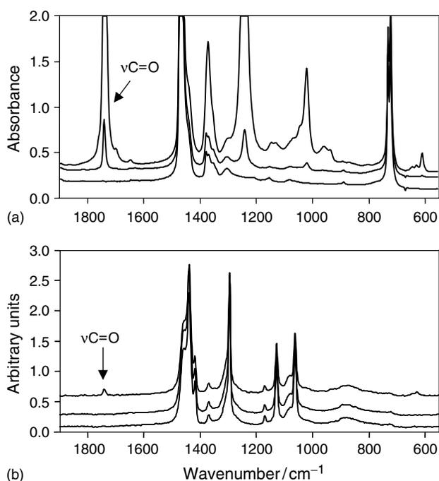
**Figure 22.** (a) IR absorbance and (b) Raman spectra recorded from two EVA copolymers containing 7.7% and 0.65% VA, and an LDPE. The LDPE spectrum is the lower in each series; the higher VA content copolymer is the uppermost spectrum in each set.
