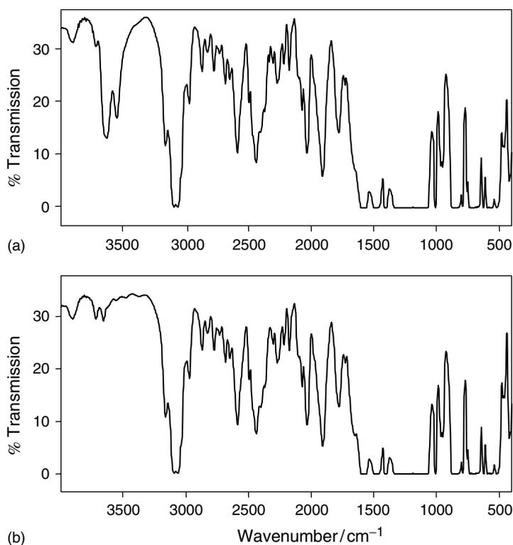
**Figure 12.** IR transmission spectra recorded from a PES film (a) before and (b) after drying.
