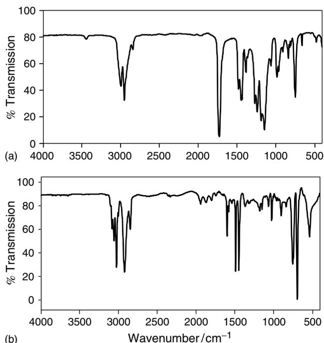
**Figure 23.** IR transmission spectra of (a) PMMA and (b) polystyrene.
