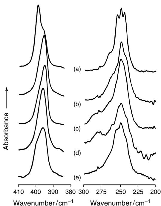
**Figure 19.** Far-infrared spectra recorded from various polymorphs of i-PP at 100 K: (a) highly crystalline  $\alpha$  i-PP; (b) quenched (amorphous)  $\alpha$  i-PP; (c)  $\beta$  i-PP; (d) "smectic" i-PP; and (e)  $\gamma$  i-PP. [Reproduced from D.R. Beckett *et al.*, *Eur. Polym. J.*, **21**, 849 (1985) by kind permission of Elsevier Science.]
