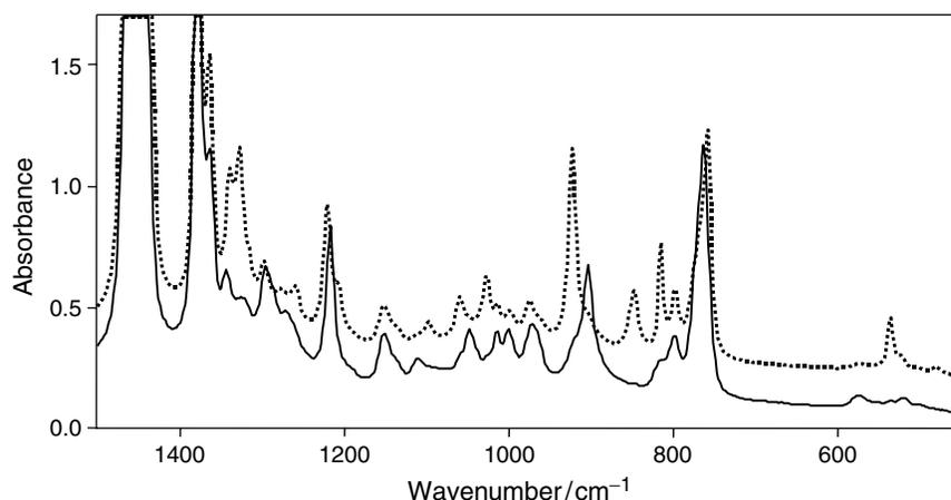
**Figure 18.** IR absorbance spectra recorded from type I (dashed line) and type II (solid line) polybutene. See text for details.
