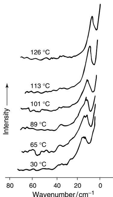
**Figure 20.** LAM Raman spectra of a PE sample. The PE was originally quenched in ice water and subsequently annealed for 1 h at a series of temperatures. [Reproduced from J.L. Koenig and D.L. Tabb, *J. Macromol. Sci.–Phys.*, **B9**, 141 (1974) by courtesy of Marcel Dekker, Inc.]
