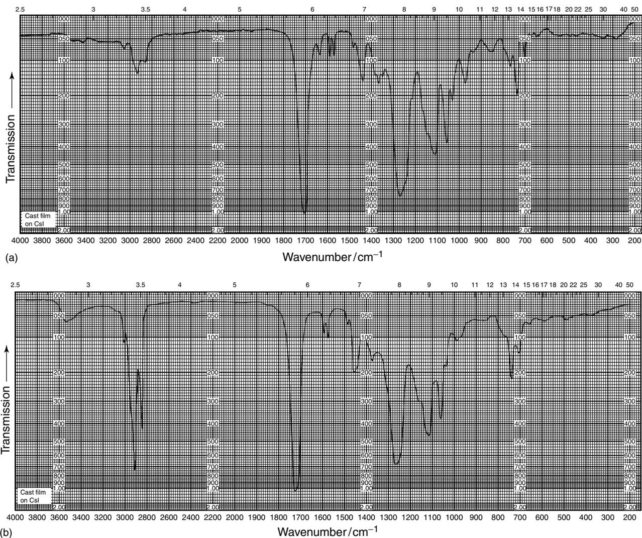
**Figure 8.** IR transmission spectra of (a) a polyester polymer based on  $\sigma$ -phthalic anhydride (40.8%), maleic anhydride (21.1%), propylene glycol (17.9%) and diethylene glycol (20.2%), and (b) a long oil alkyd based on  $\sigma$ -phthalic anhydride (24%), soybean oil (61%) and glycerine (15%). [Reproduced from spectra numbers 300 and 96, respectively, in ‘An Infrared Spectroscopy Atlas for the Coatings Industry’, Federation of Societies for Coatings Technology, Pennsylvania (1980).]
