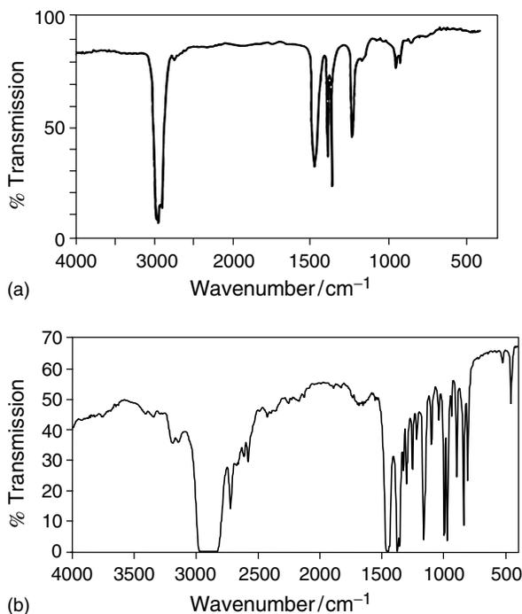
**Figure 4.** IR transmission spectra of (a) PIB and (b) isotactic polypropylene (i-PP).
