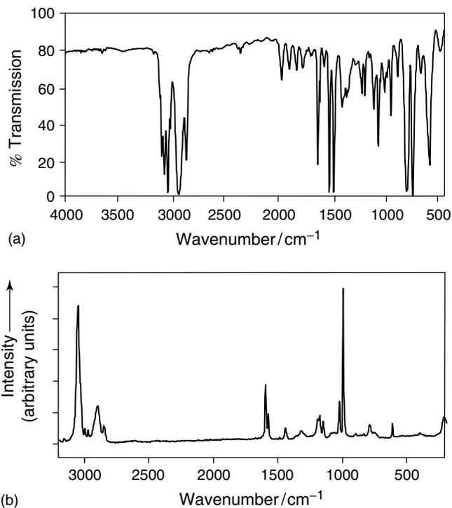
**Figure 5.** (a) IR transmission and (b) Raman spectra of polystyrene.
