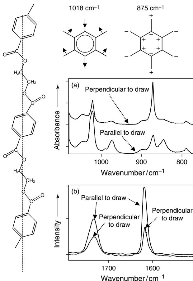
**Figure 16.** PET orientation: schematic of an oriented PET chain, and IR active modes at  $1018\text{ cm}^{-1}$  and  $875\text{ cm}^{-1}$ , and polarized (a) IR absorbance and (b) Raman spectra recorded from a uniaxially oriented PET. Parallel and perpendicular refer to the alignment of the electric vector of the radiation with respect to the draw (chain) axis of the polymer.
