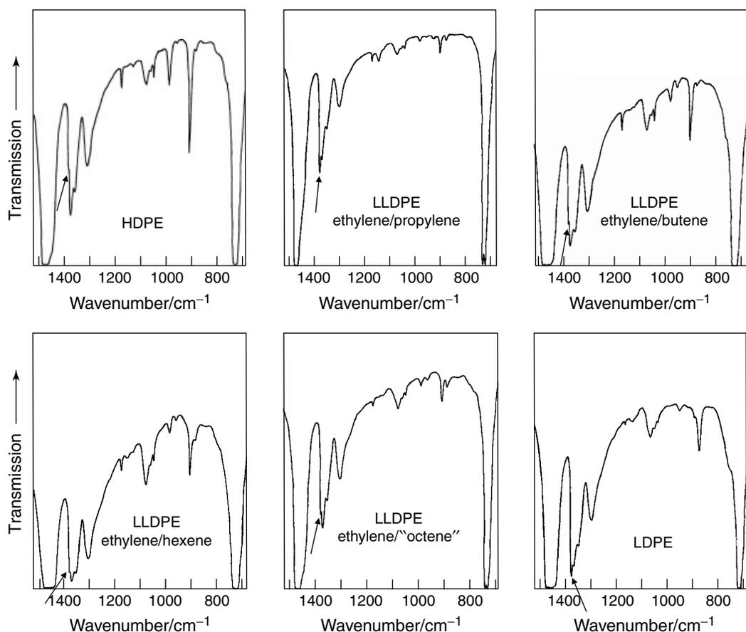
**Figure 10.** IR transmission spectra over the range  $1500$  to  $700\text{ cm}^{-1}$  recorded from films of six different commercial PEs: HDPE; LDPE; and LLDPE, linear low-density polyethylene. The  $\alpha$ -olefin copolymer determined by NMR is labeled for each LLDPE. For the figure labeled “octene” this signifies ( $\geq$ )octene, as the chain length determined from the NMR measurement. The arrows indicate the position of the  $\delta_{\text{sym}}\text{ C-CH}_3$ .
