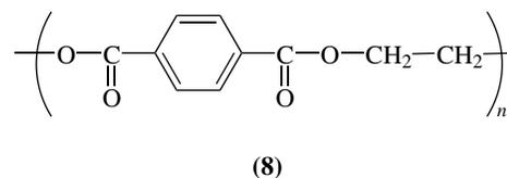
In accord with its structure, the IR and Raman spectra each show a  $\nu\text{C}=\text{O}$  band at  $\sim 1725\text{ cm}^{-1}$ , and the IR spectrum shows very strong  $\nu\text{C}-\text{O}$  bands at  $\sim 1250\text{ cm}^{-1}$  and  $\sim 1100\text{ cm}^{-1}$  that are characteristic of an aromatic ester. Aromaticity is confirmed in the IR spectrum by the sharp ring stretching bands near  $1600$ ,  $1500$  and  $1450\text{ cm}^{-1}$ , and
