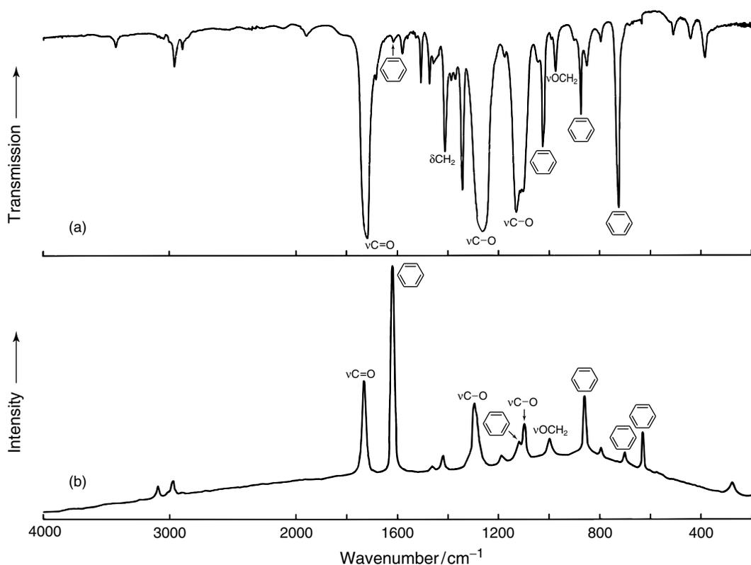
**Figure 7.** (a) IR transmission and (b) Raman spectra of PET. [Reproduced, with permission, from H.A. Willis, 'Combination of Spectroscopic Methods in Polymer Structure Analysis', in "Proceedings of 5th European Symposium on Polymer Spectroscopy", ed. D.O. Hummel, Verlag Chemie, Weinheim (1979).]
