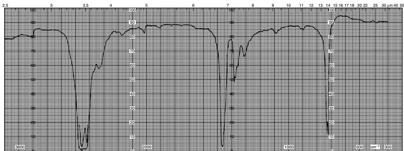
**Figure 1.** IR transmission spectrum of a low-density polyethylene (LDPE). [Reproduced from spectrum number 1916 in ‘Atlas of Polymer and Plastics Analysis’, 2nd edition, Vol. 2, Part a/I, D.O. Hummel, Verlag Chemie, Weinheim (1984).]
