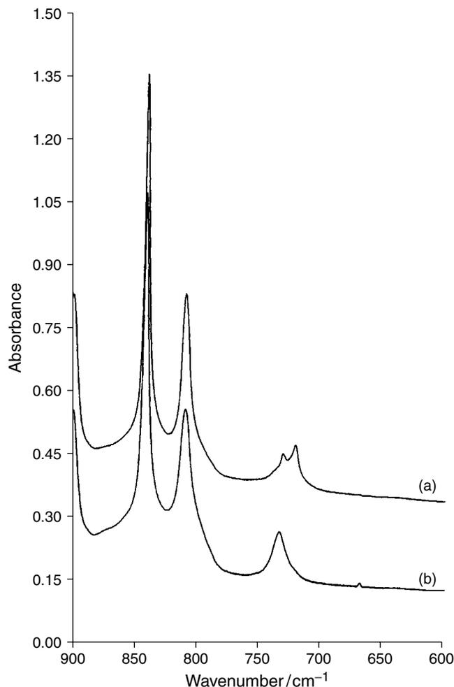
**Figure 25.** IR absorbance spectra over the range 900 cm<sup>-1</sup> to 600 cm<sup>-1</sup> recorded from films prepared from propylene/ethylene copolymers containing ~5% copolymerized ethylene: (a) a “block” copolymer containing long -(CH<sub>2</sub>)- sequences; (b) a “random” copolymer containing essentially only isolated ethylene units.
