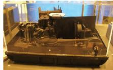
To the left is the prototype of the first commercial IR spectrometer, the Beckman IR-1. The story of this instrument, told by its designer, R.R. Brattain, can be read at <a href="http://www.s-a-s.org/epstein/WWII/index.html/">http://www.s-a-s.org/epstein/WWII/index.html/</a>.
