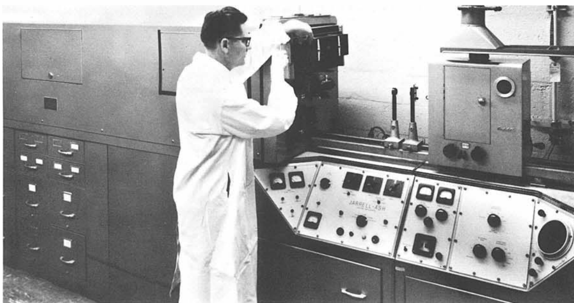
A. M. Liebman, Supervisor of Spectrographic Laboratory, operates the JACO 3.4-Meter Ebert spectrograph. Above, he is shown pulling dark slides from plate holder; right, running a sample.
