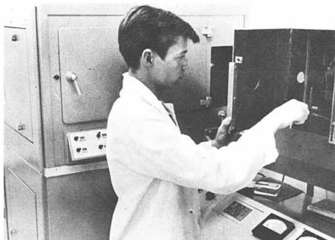
Laboratory Assistant, Paul Bouchard, lines up electrodes for optical emission examination of a high purity metal.
