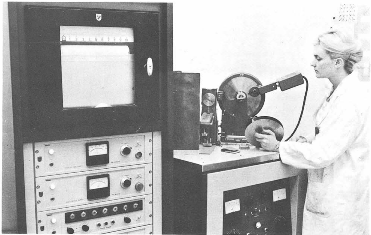
Crystallographer, Marthe Beaudry, sets the goniometer for x-ray diffraction examination of a concentrate.
