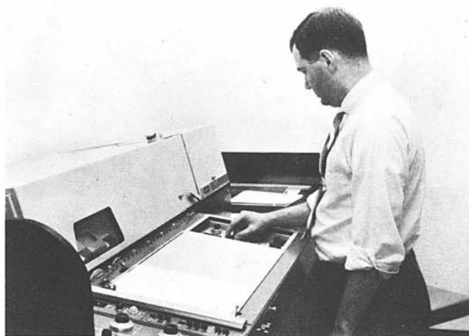
Spectroscopist, Ken Lea, determines trace amounts of carbon in high purity selenium by the infrared technique.
