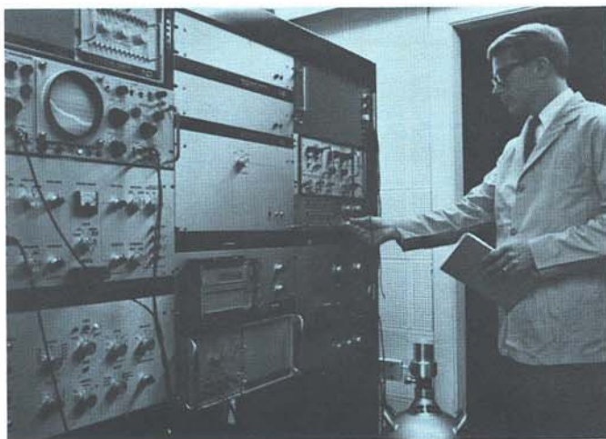
FBI Agent operating multichannel analyzer and solid state detector used for gamma ray studies in conjunction with analyses by neutron activation.
