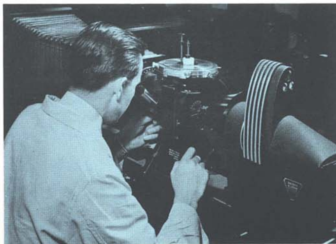
In the metallurgy unit of the FBI Laboratory the metallograph is used to study the crystalline structure of metals.
