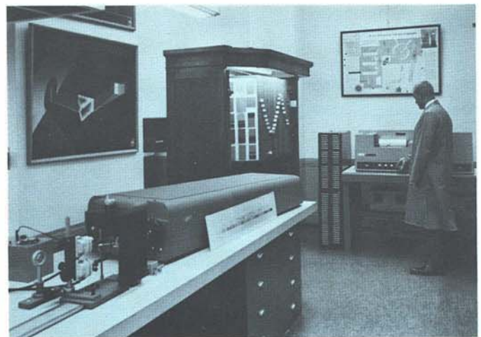
Ultraviolet, visible and near infrared spectrophotometer examination being conducted by FBI Laboratory technician. 1.5 meter emission spectrograph and FBI National Automotive Paint File at left.
