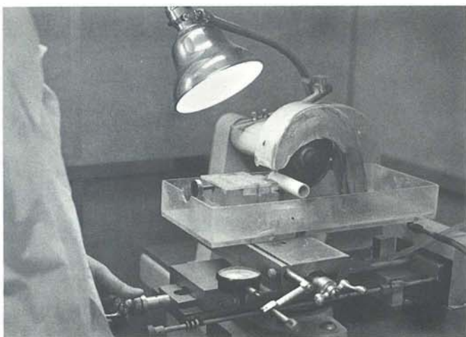
Cutting specimens for preparation of thin and polished sections prior to photomicrographic examination.
