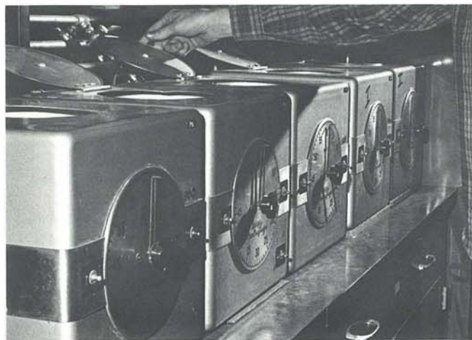
Particle Size Distribution of powders by the Whitby Centrifuge accelerated gravity technique.
