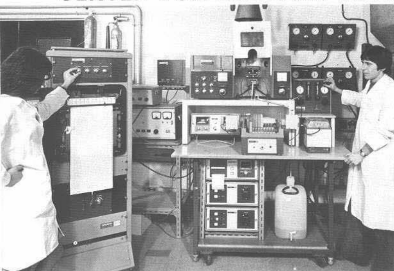
Christabel Picca and Andre Mayol utilize atomic absorption spectroscopy for metal trace determinations in solutions.
