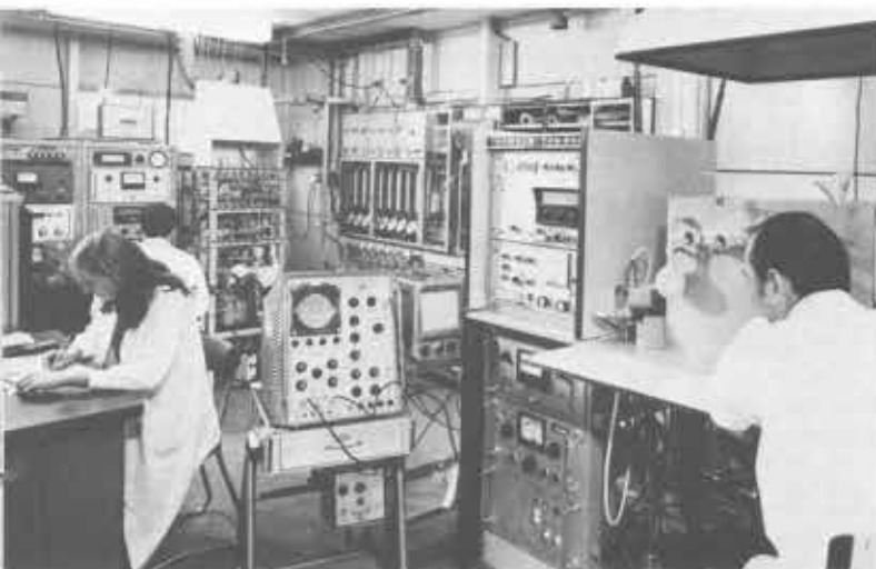
With on-line mass spectrometer output data, Adriana Godard is computing precise deuterium content of effluents flowing from the pilot plant for French heavy water producing process.
