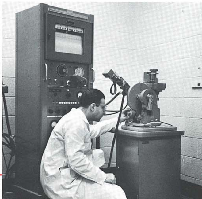
MR. S. BOGDAN, in charge of emission and X-ray facilities, adjusts angle on wide range goniometer for fluorescence measurement.
