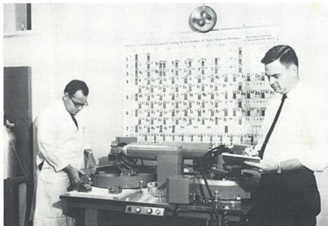
MR. AL BIGATEL (left) Engineering Associate of the production laboratory, and Mr. Bob Ramsey, Engineer of the development laboratory are using the General Electric Company XRD-5 X-ray spectrometer with the Heinrich miniature probe to identify metallic particles 0.005 inches in size separated from an electron tube mixture.
