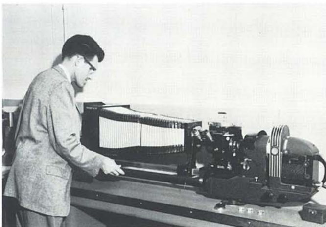
MR. TOM BRIGGS, development engineer, of the development chemical laboratory is making an adjustment to the camera of the Bausch & Lomb research metallograph prior to taking a micro-photograph of the structure of a semi-conductor device.
