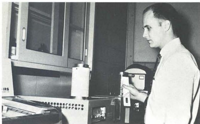
Dr. Robert Evers, Organic Research Chemist in the Polymer Branch, monitors recording of infrared spectrum of a high-temperature polymer on a Perkin-Elmer Model 137 Infrared "Infracord" Spectrophotometer.
