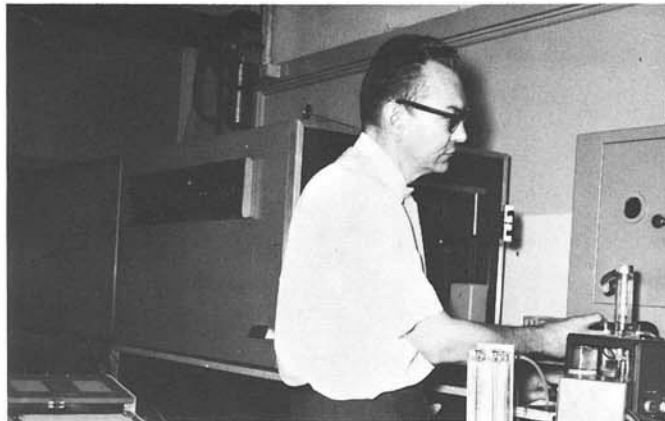
Research Chemist James Muntz using the ultrasonic nebulizer for quantitative analysis of research materials on the Jarrell-Ash 3.4 meter emission spectrograph.
