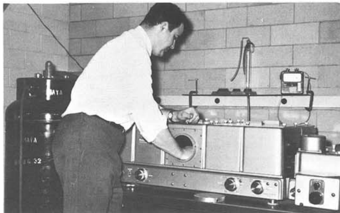
Research Chemist Neil McDevitt places sample of material in the compartment of Perkin-Elmer Model 301 Spectrophotometer preparatory to analysis of the substance. The tank at the left contains liquid nitrogen which is necessary in the maintenance of the instrument.
