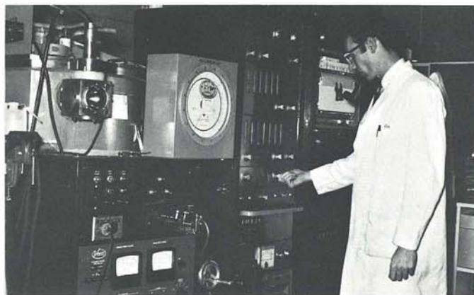
Physicist Dave Fisher adjusts controls on Picker Soft X-Ray Spectrometer. The study of X-ray emission and absorption spectra contributes greatly to the basic research in the physics of spectra.
