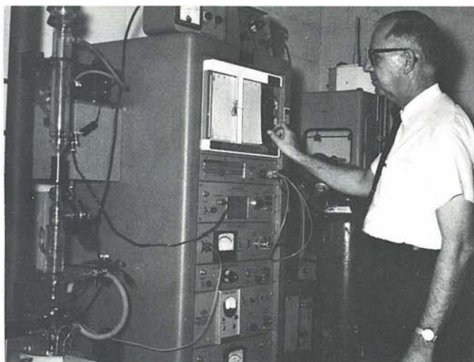
Charles Houston, Supervisory Chemist, Activates thermogravimetric recording instrument which measures changes in the weight of a substance as a function of temperature. This instrument supports research in the Ceramics and Graphite Branch.
