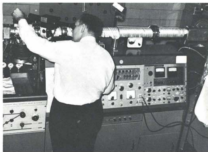
Scientist Edmund Rolinski examines material preparatory to a high-temperature investigation of binary and ternary titanium alloys on the Bendix TOF Mass Spectrometer. This instrument supports research in the Thermo and Chemical Physics Branch and Advanced Metallurgical Studies Branch. (Continued on Page 10)
