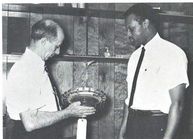
Physical Metallurgists George Yoder and Russell Henderson inspect a first-stage titanium alloy compressor disc from an aircraft to be analyzed for possible defects.
