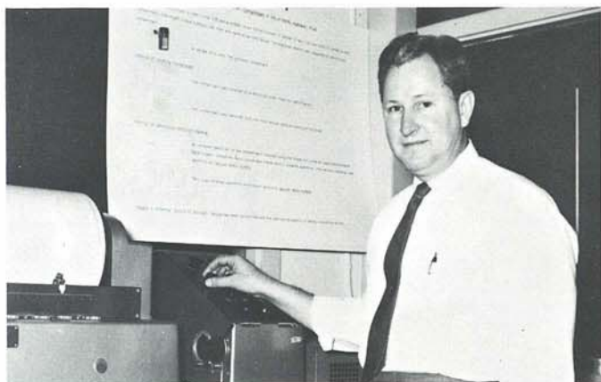
Freeman F. Bentley, Chief of the Analytical Branch of the Materials Physics Division, Air Force Materials Laboratory, adjusts controls on Perkin-Elmer Model 21 Recording Infrared Spectrophotometer as he attempts to identify an unknown organic compound by its long wavelength infrared spectrum. This particular spectrophotometer, built to the specifications of the AFML research chemists in 1954, is the first double beam instrument to record spectra in the 15-35u region.
