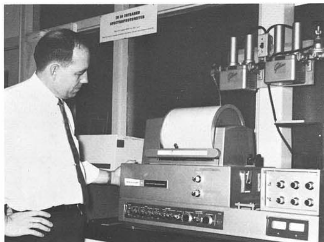
Chemist Bill Crawford observes graphic record produced on Perkin-Elmer 521 Grating Infrared Spectrophotometer. The Spectrogram provides data useful in identification of unknown materials.
