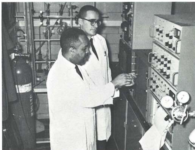
Captain Ronald Lewis and Wilbert Powell, Research Chemists, check operation of F & M Corp. Model 5750 Analytical Gas Chromatograph which accomplishes the separation of organo-metallic materials and also identifies and characterizes materials.
