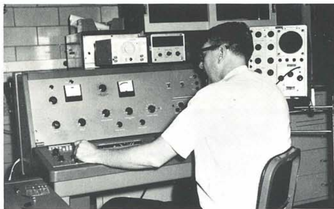
Dr. Dan Dyer, Research Chemist, adjusts controls on console of Varian A-56/60D Nuclear Magnetic Resonance Spectrometer which characterizes organic and organo-metallic materials containing protons and/or fluorine -19 nuclei.
