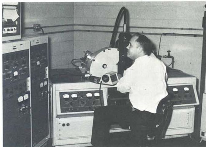
Dr. C. T. Lynch, Senior Scientist, operates Electron Microprobe Analyzer which discerns segregation of impurities in alloys. The readout emerging at the left is recording the concentrations in yttrium.
