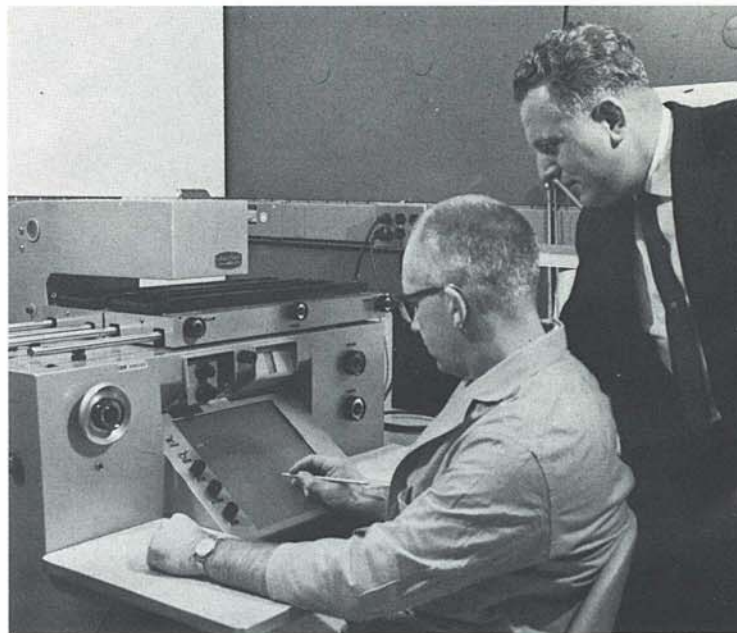
MR. WEBBER, at the microphotometer, consults Dr. Reuter regarding a new technique for estimation of gap temperatures.
