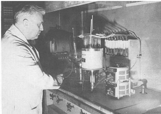
OPERATING the Wocot Lubricating Oil Oxidation test apparatus is Chief Chemist Herb Wochele. Mr. Wochele assisted in originally developing the test.
